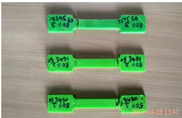
Fig 13 Fractured specimens at 50% Infill density
