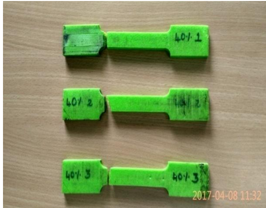
Fig 12. Fractured specimens at 40% Infill density
